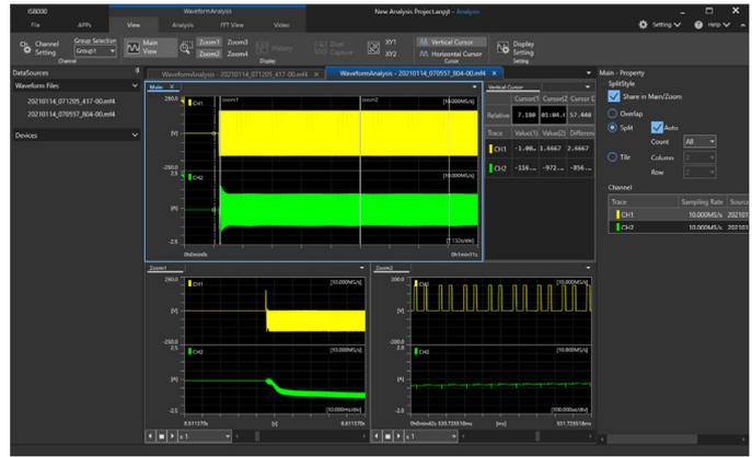
Figure 3. 10 MS/s data transfer measurement screen from DL 950
