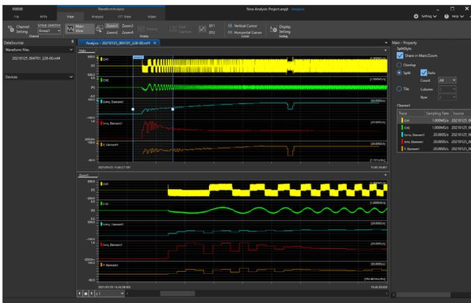
Figure 5. Time-synchronized display of power data and waveform data
