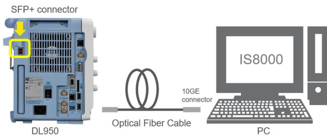
Figure 2. Connection between DL950 and PC
