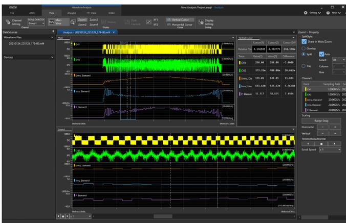
Figure 6. Cursor measurement of power data and waveform data
