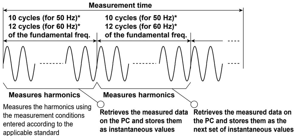
One set of harmonic measurement data (handled as instantaneous values by the software) consists of harmonic data measured every 200 ms (10 cycles for 50 Hz and 12 cycles for 60 Hz)\*. The instantaneous values, the mean value, and the maximum value of the measured data retrieved within the measurement time (see next page) can be evaluated to determine whether they are within the limits of the standard.
