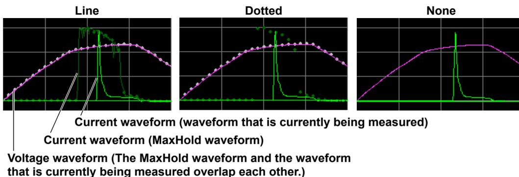
When MaxHold is set to Dotted or Line, the measured value of wave judgment takes on the following value.
