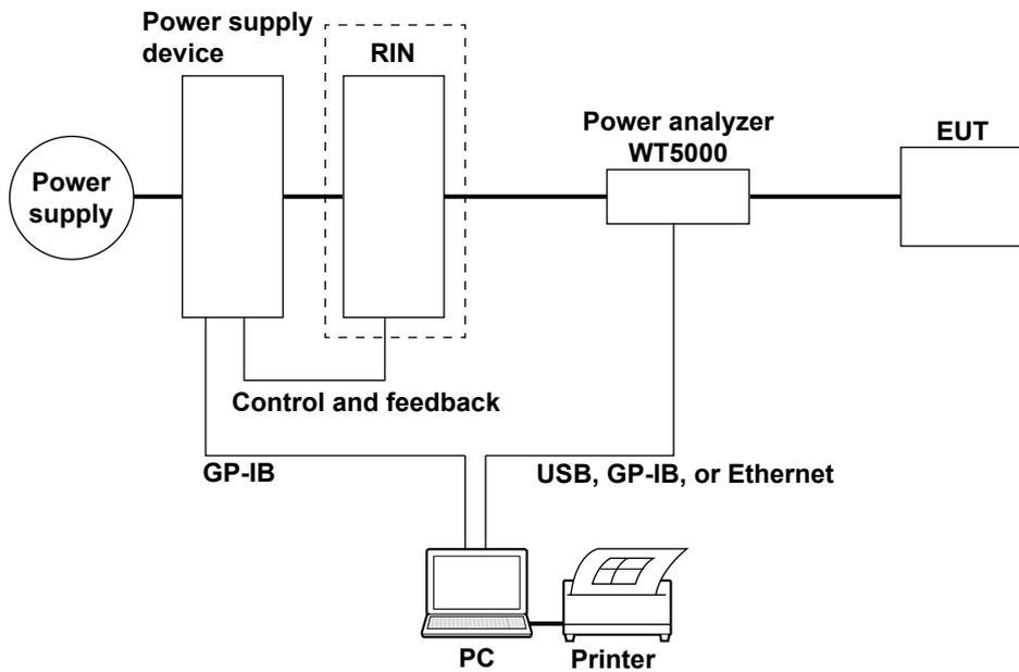
To use the power supply control function, connect the NF power supply to the PC via GP-IB.
