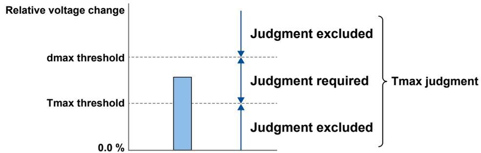
If Tmax is added to the judgment, a Ztest/Zmax check is performed to verify whether the Tmax threshold is appropriate. If it is inappropriate, the Tmax threshold is updated, and measurement is performed again.
