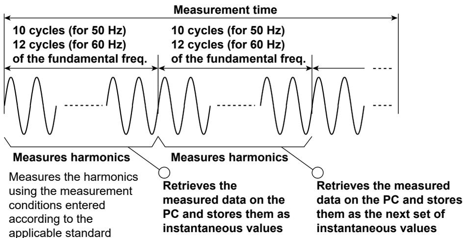
For IEC 61000-4-7 Edition 2.0 or Edition 2.0 A1, one set of harmonic measurement data (handled as instantaneous values by the software) consists of harmonic data measured every 200 ms (10 cycles for 50 Hz and 12 cycles for 60 Hz). The instantaneous values, the mean value, and the maximum value of the measured data retrieved within the measurement time (see next page) can be evaluated to determine whether they are within the limits of the standard.
