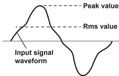
The crest factor on the WT is determined by the maximum peak value that can be applied for rated input in terms of a multiplication factor.
