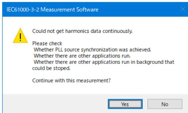
This software retrieves large amount of measured data from the WT. The error message may appear if the CPU on the PC is overloaded and cannot keep up with the data transfer. Lighten the load placed on the CPU on the PC by checking the points listed below.
