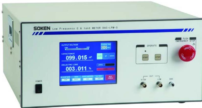
Model DAC-LFM-3 is designed to measure tan  $\delta$  and capacitance of test samples by making use of a built-in very-low frequency power source.
