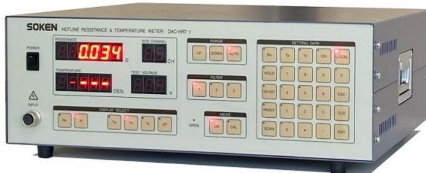
DAC-HRT-1 is designed for temperature rise tests of motors, transformers, coils, chokes and etc, under energizing AC voltage. The direct reading of resistance is possible with 4-terminals measurement method, and temperature is automatically calculated from measured resistance values and displayed.
