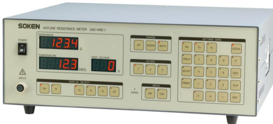
DAC-HRE-1 is designed for temperature rise tests of motors, transformers, coils, chokes and etc, under energizing AC voltage. The direct reading of resistance is possible with 4-terminals measurement method, and temperature is calculated from measured resistance values and displayed.
